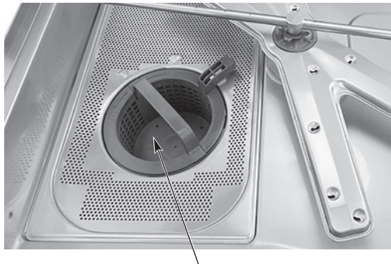
STRAINER BASKET IN UNLOCKED POSITION
